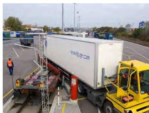
Figure 13: Wagon platforms can swivel to allow loading/unloading
