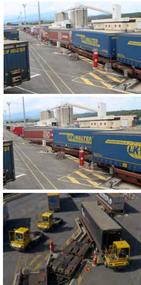
Figure 6: Piggyback rail in Europe - wagons being discharged at Le Boulou terminal, south of France
