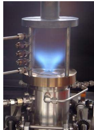
Figure 4. Detail of DLR's combustion chamber.
