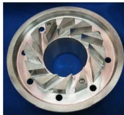
Figure 6. Swirler detail without the central cone.
