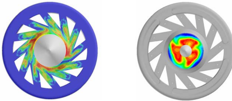
Figure 21. Laminar flame velocity contour displayed inside swirler and injector.
